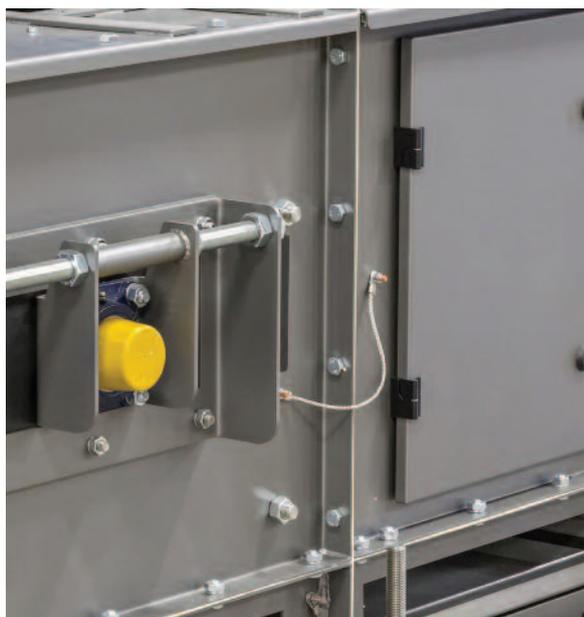
**Using grounding or earthing straps and implementing gasketing between sections and around access doors helps create an air-tight seal on a bucket elevator**
