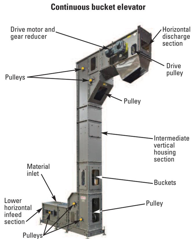
specially shaped buckets that are joined together to hold material during the vertical and horizontal transfers.) Buckets then tip to empty only at the elevator's discharge point. The buckets interlock or overlap to prevent spillage during continuous material infeed, and the elevator design can be open, enclosed, or fully sealed to prevent material contamination or avoid emissions being released.
